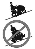
Do not mow across slopes when using under or rearmount mowers
